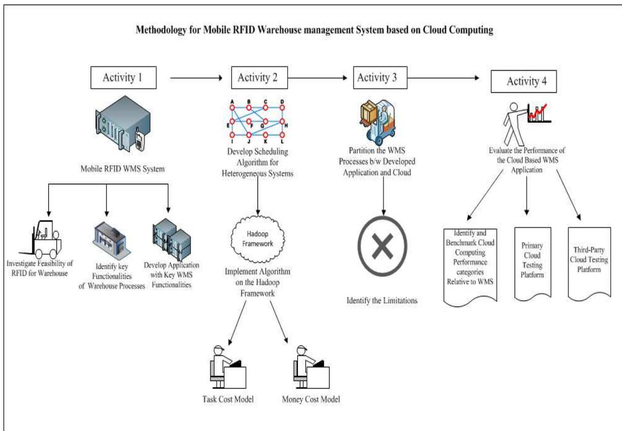
**Figure 3.** Methodology for Mobile RFID Warehouse Management System based on Cloud Computing
