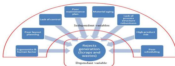
**Figure 3:** The factors resulting in increasing scraps and wastes at production shop-floor
